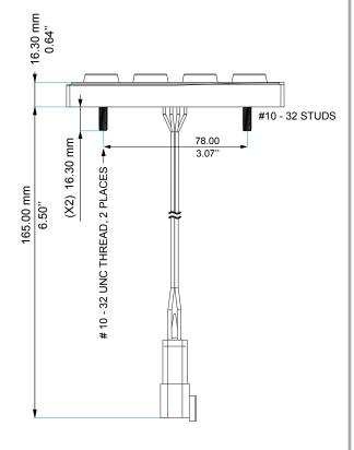
MOUNTING NOTES: Nuts thread: #10-32 Maximum torque: 1,8Nm
