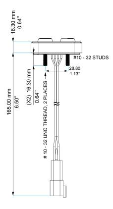
MOUNTING NOTES: Nuts thread: #10-32 Maximum torque: 1,8Nm
