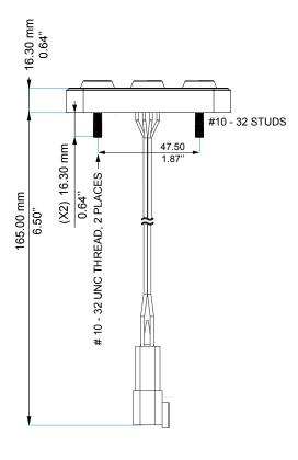
MOUNTING NOTES: Nuts thread: #10-32 Maximum torque: 1,8Nm
