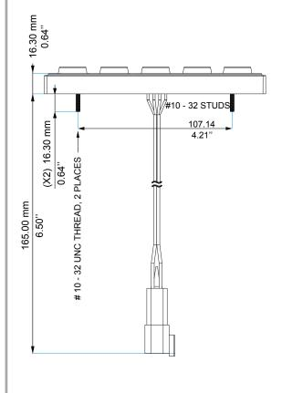
MOUNTING NOTES: Nuts thread: #10-32 Maximum torque: 1,8Nm
